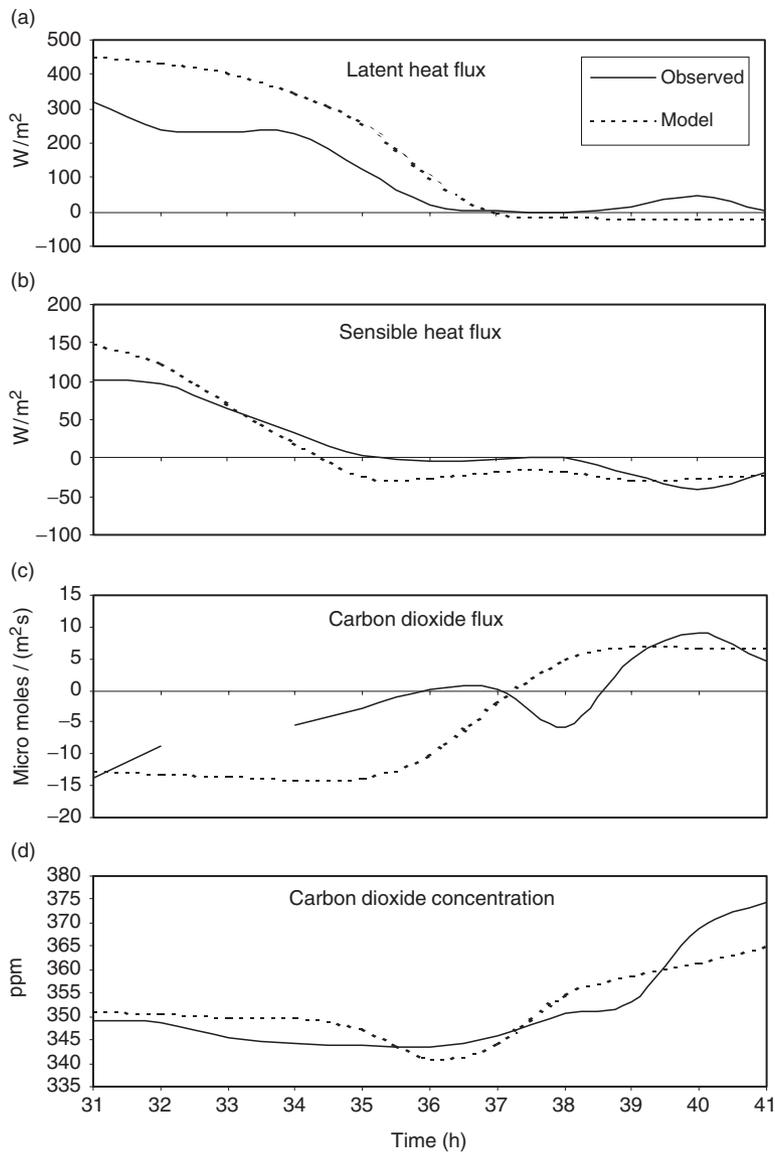
**Fig. 7** Analysis of the evening transition on July 27, showing the early development of the stable layer in SiB-RAMS which was not observed. (a) Latent heat flux, (b) sensible heat flux, (c) carbon dioxide flux, and (d) carbon dioxide concentration at 30 m above ground. Time is elapsed time since the beginning of the experiment, in hours ( $t = 31$  corresponds to 13:00 hours LST on July 27).
