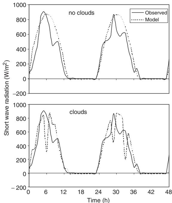
**Fig. 1** Simulated and observed downward solar radiation for July 26–27, 1997. Simulations used the high-resolution, two-dimensional grid. The upper panel is for cloudless conditions, and the lower panel shows results including passing clouds. Time is elapsed hours since the beginning of the experiment at 06:00 hours LST on July 26, 1997.
