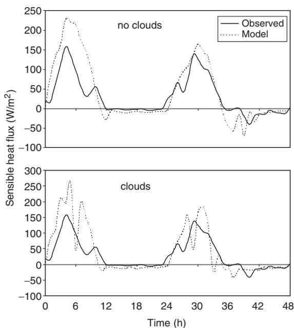
**Fig. 2** Simulated and observed sensible heat fluxes for July 26–27, 1997, at 30 m. The upper panel is for cloudless conditions, and the lower panel shows results including passing clouds. Time is elapsed hours since the beginning of the experiment at 06:00 hours. LST on July 26, 1997.
